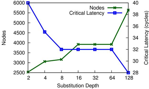
Fig. 3: Node and critical path latency trends with increasing depth-limited substitution (*bomhof2*)
