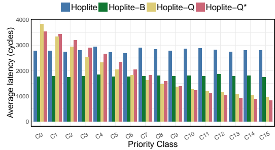
Figure 8: Average latency suffered by packets in each priority class for 8 \times 8 NoC, where C = 16 and P = 8 .
