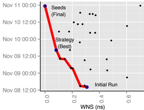
Fig. 3: Worst-Case Negative Slack improvements vs. time for UDP offload engine. *Strategy* is the machine-learning driven improvement in WNS scores, *Seeds* if the final seed exploration to mop up remaining slack.
