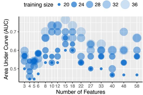
Fig. 9: Impact of Feature Size on AUC trends for varying Training Set sizes for the *net\_chn4* benchmark. Balloon sizes correspond to training size. Too few features < 8 result in low AUC scores of 0.5–0.6. Too many features result in a dropoff in AUC scores again. *Goldilocks* range of features 8–22 deliver high AUC scores of 0.7–0.8.
