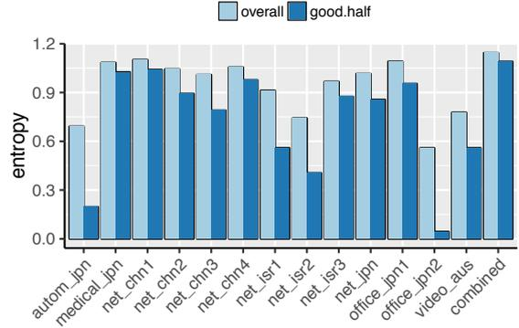
Fig. 6: Entropy of the explored CAD parameter combinations and the dissimilarity of optimal parameter combinations needed for timing convergence (column combined). `overall` corresponds to all CAD runs, while `good.half` corresponds to the TNS-improving combinations.
