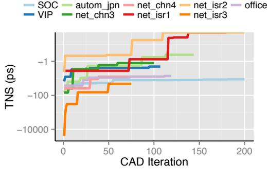
Fig. 5: TNS convergence of various benchmarks with InTime (logscale  $y$ -axis, most designs with non-zero TNS scores still converge in a final seed exploration cleanup phase).
