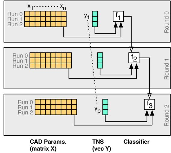
Fig. 2: Various steps of building and improving the classifier  $f_r$  in each learning round  $r$ . Multiple parallel CAD iterations are organized into *rounds*. Results from a round are collected together and used to updated the classifier function  $f_r$ .
